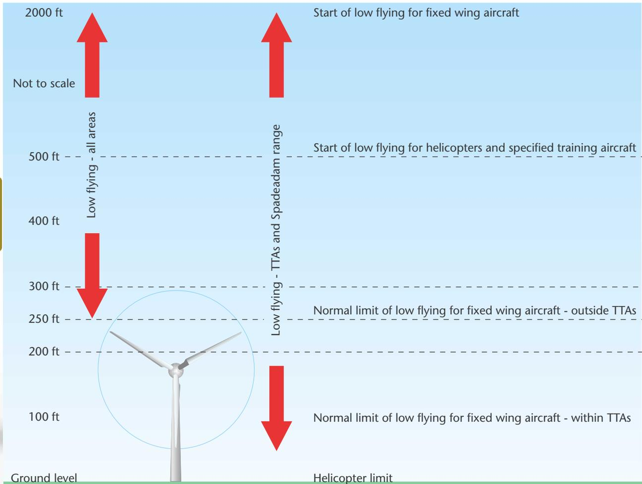
**Figure 3-2.** Comparison of Low Flying Limits with 80m Rotor Diameter Turbine
