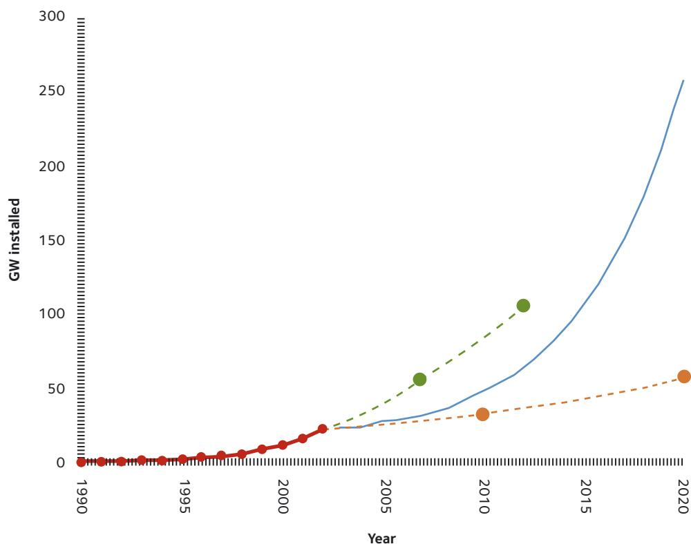
720TWh/year is equivalent to approximately 240GW of offshore wind capacity. Figure 2.2 below postulates a growth pattern for this amount of offshore wind power (the blue line), which is shown as an extension from the present-day installed capacity of on- and offshore wind (the red line). The same figure also shows trend lines fitted to the IEA's OECD Europe baseline (in orange) and BTM's predictions (in green) for on- and offshore wind power.
