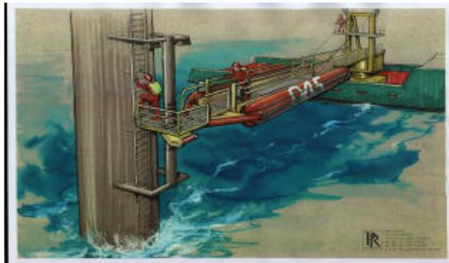
• **Figure 4:** Offshore Access system using a flexible gangway
