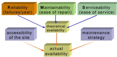
**Figure 2:** Availability as function of machine properties, site accessibility and maintenance strategy
