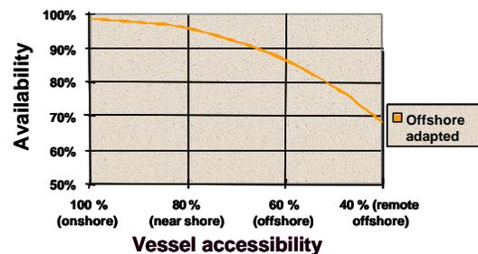
**Figure 3:** Availability as function of vessel accessibility of a 100 unit offshore windfarm.
