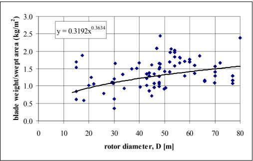
Figure 2.9 Rotor mass/ swept area ratio
