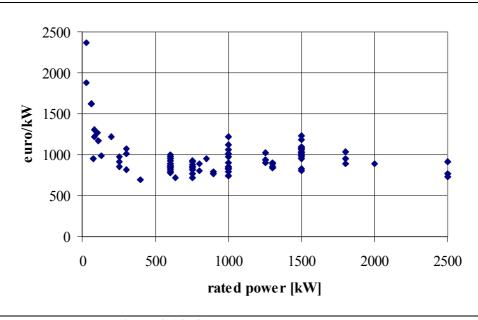
Figure 2.14 Cost per kW v rated power
