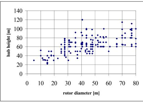
Figure 2.4 Hub height variation of wind turbines
