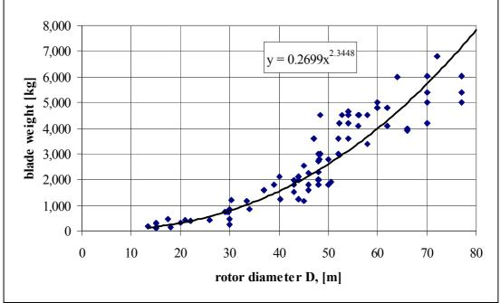
Figure 2.7 Blade mass related to rotor diameter
