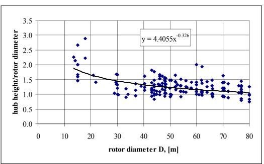
Figure 2.10 Hub height/rotor diameter ratio
