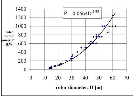
Figure 2.1 Power rating of wind turbines up to 62 m diameter
