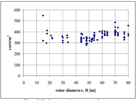
Figure 2.12 Cost per unit swept area v diameter
