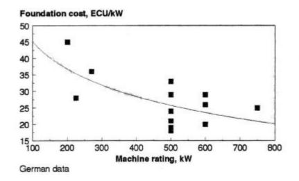
Figure 2.15 Foundation cost v rated power
