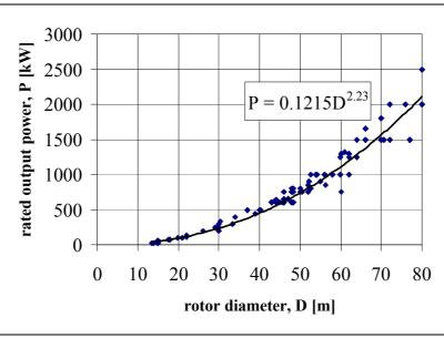
Figure 2.2 Power rating of wind turbines
