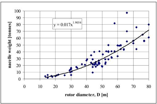
Figure 2.8 Nacelle mass v rotor diameter
