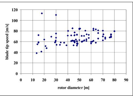
Figure 2.3 Design tip speed (maximum steady state)
