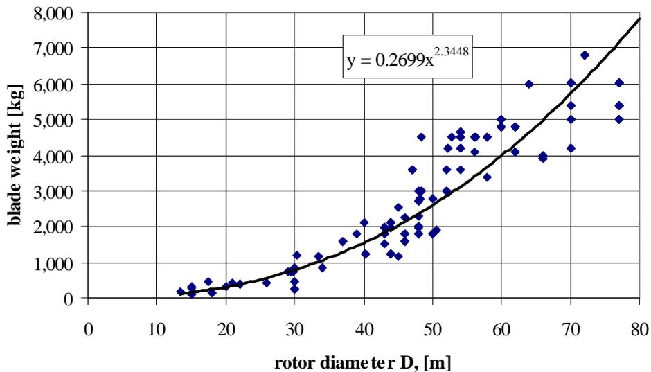
**Figure 2.1.3.3 Blade mass related to rotor diameter**
