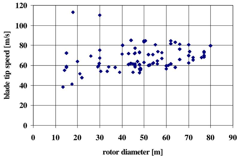
Figure 2.1.2.3 Design tip speed (maximum steady state)
