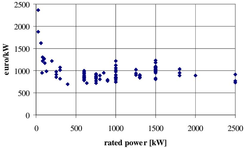
**Figure 2.1.4.4 Cost per kW v rated power**
