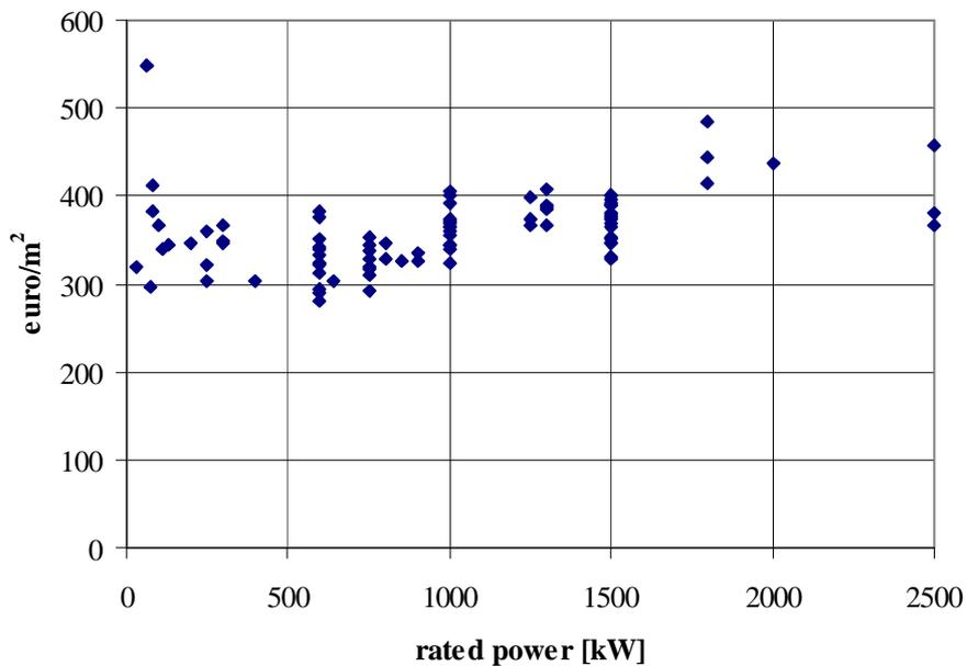
**Figure 2.1.4.3 Cost per unit swept area v rated power**
