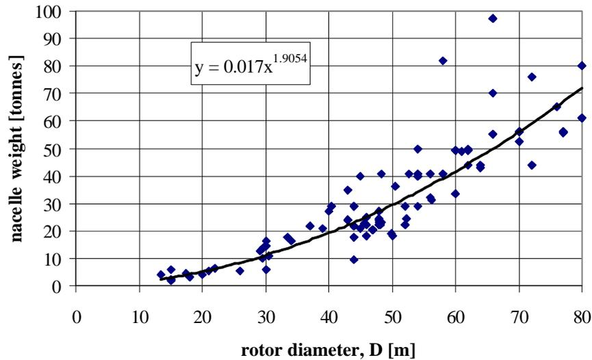
**Figure 2.1.3.4 Nacelle mass v rotor diameter**
