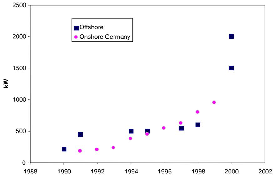
Figure 2.1.3.1 Rating trends in land based and offshore wind turbines
