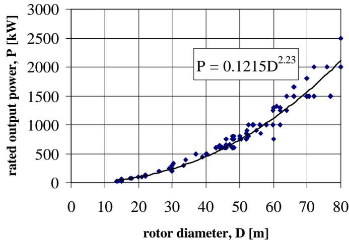
Figure 2.1.2.2 Power rating of wind turbines
