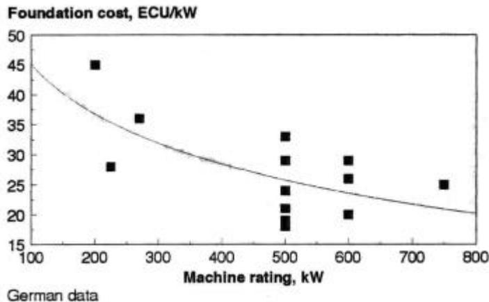
**Figure 2.1.4.5 Foundation cost v rated power**
