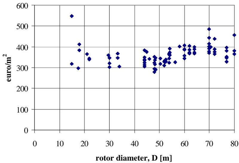
**Figure 2.1.4.2 Cost per unit swept area v diameter**
