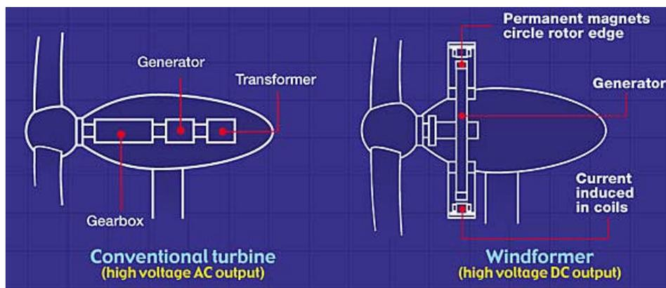
**Figure 7.1.3.1** Diagram comparing conventional and Scanwind concepts
