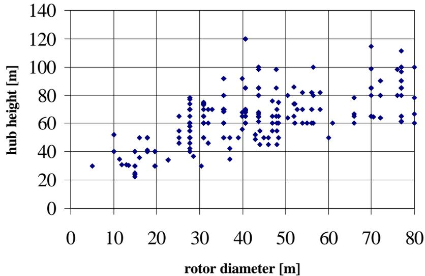
**Figure 2.1.2.4 Hub height variation of wind turbines**
