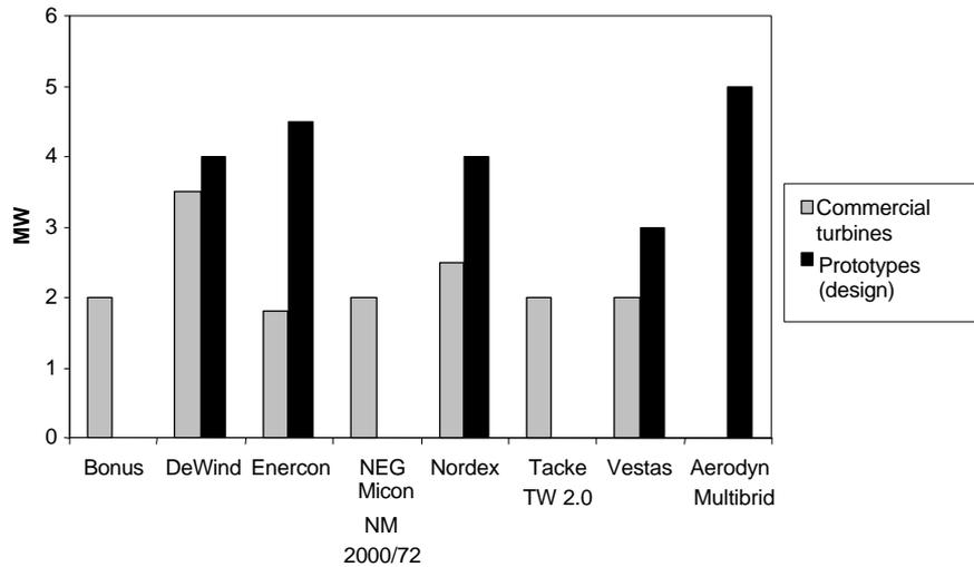
**Figure 2.1.3.2 Commercial offshore turbines and forthcoming prototypes**
