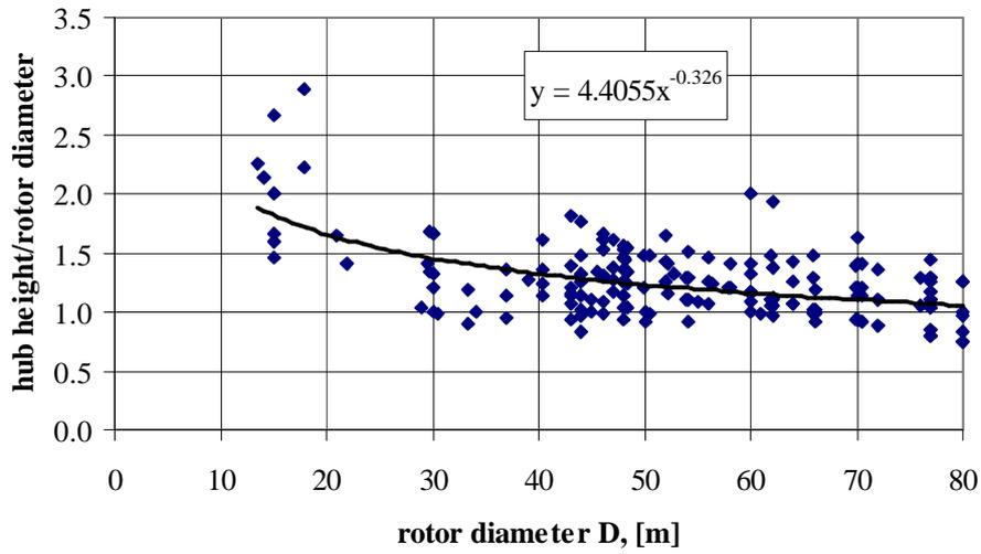
Figure 2.1.3.6 Hub height/rotor diameter ratio
