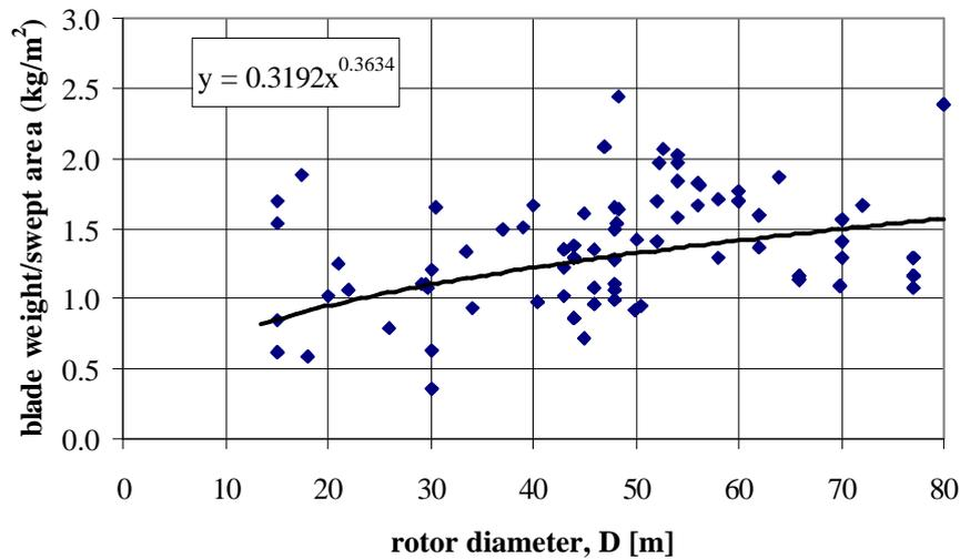
**Figure 2.1.3.5 Rotor mass/ swept area ratio**
