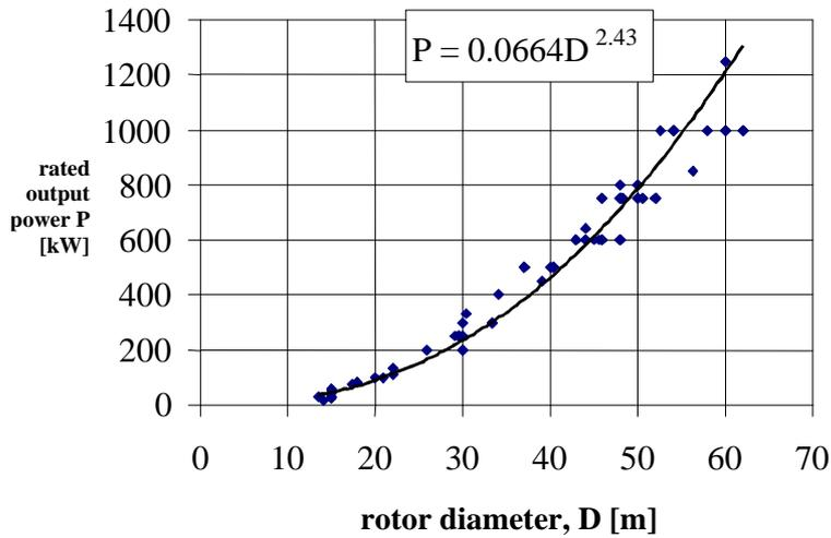
Figure 2.1.2.1 Power rating of wind turbines up to 62 m diameter
