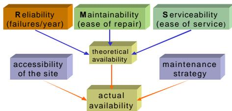
**Figure 2:** Availability as function of machine properties, site accessibility and maintenance strategy
