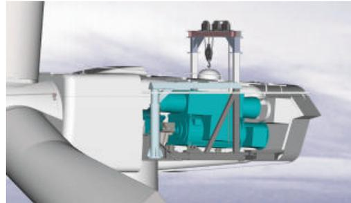
**Figure 5:** Built in crane for exchange of nacelle components. Enron 1,5S Offshore wind-turbines at Utgrunden, SE.
