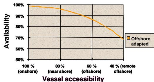
**Figure 3:** Availability as function of vessel accessibility of a 100 unit offshore windfarm.
